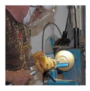
This vibration can be avoided by simply lifting the bevel slightly (and not pressing so hard). When making a final smoothing cut, bumps do not matter as they can be sanded off readily but "pick out" is a problem as much more wood needs to be sanded-off. For final smoothing cuts Terry uses the bowl gouge on the side with the lower flute just touching the wood to get a smooth clean finish.
