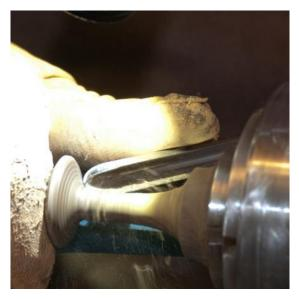
showed how he makes a secondary tenon on the base of his turnings that creates some extra wood between the chuck and the base of the item. This extra wood can be parted off with a thin parting tool which then makes it relatively easy to complete a smooth base.
