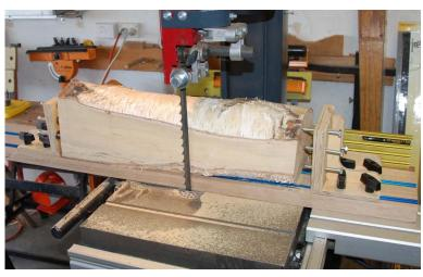
**Green Wood:** A general rule is that green timber should not be cut using the bandsaws, as wet wood tends to gum up the blade and wheels, which are then difficult to clean. A benefit of this log jig, however, is the ability to cut thin boards from a green log so they can season in 6 to 12 months, rather than having to wait years for a log to dry that may by then be rotten or split.
