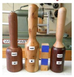
These two mallets are the shape and size I now believe to be the most efficient for a Tapping Mallet. The Chinese Elm mallet is 235mm in length, while the Gidgee mallet is 230mm. The separate dense Gidgee head with a lighter handle gives a quite different balance.
