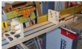
the flat side on the bottom, and a second cut made at right-angles. This provides two faces at right-angles, as seen at right below, so that a series of boards of a set width can then be cut, using the normal fence with the jig removed.
