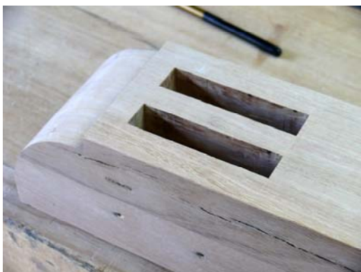
The mortices in one of the trestle sled feet.
