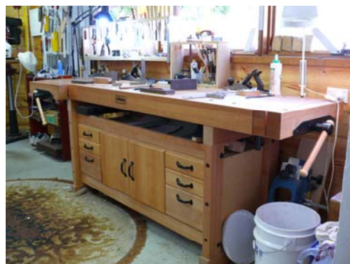
A couple of views of Justin McCarthy's workbench. Solid (indestructible probably) and eminently practical. Note the bench dogs, holdall and the ample storage space.
