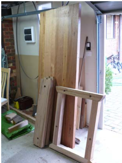
The finished top and other frame members after planing and sanding.
