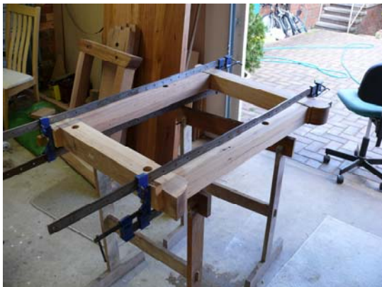
A view of the clamping for gluing of one of the frame ends. Note the holes for the connecting bolts have been drilled prior to assembly.
