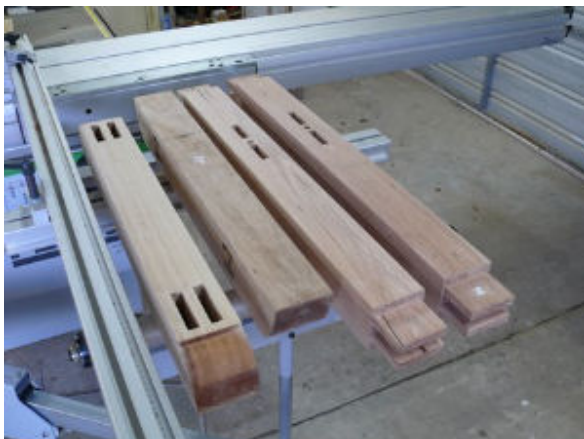
Mortice and Tenon Joints on the frame and legs
