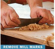
A scraper is ideal for cleaning up light tearout and marks from jointers, planers, and handplanes.
