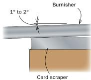
Use the burnisher at an angle of 1° to 15° to flatten this ridge and create a hook-shaped cutting burr. A steeper angle yields a more aggressive cut.
