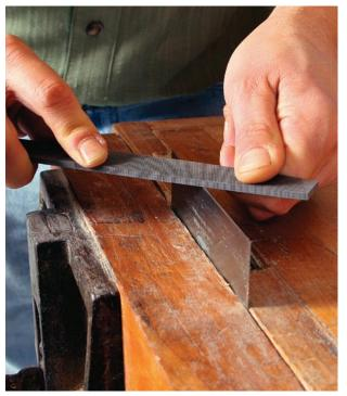
finish cut, I sometimes move on to 400 or even 600 grit. These filing and flattening steps build up a "wire edge" of thin and brittle waste material that must be removed. To do this, hold the face of the scraper at 90° to the stone or sandpaper and work the edge using light pressure. It's easier to maintain
