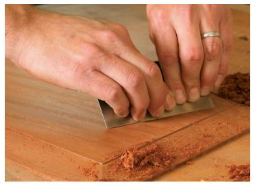
**Pulling leaves a flatter surface.** Align your fingertips behind the cutting edge to apply uniform pressure.
