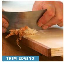
The cut is adjustable enough to trim solid edging flush and avoid damaging the plywood veneer.
