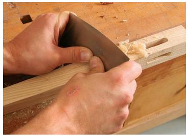
**Use caution near edges.** Avoid letting the scraper dig into the workpiece edges and leave them ragged. Here, Teague bows the scraper enough to concentrate cutting pressure in the center of the workpiece.
