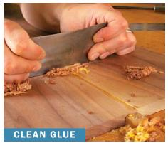
Dried squeeze-out comes off easily. Avoid an aggressive cut, which can dish the glueline.
