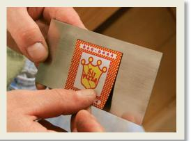
stock, I typically clean up jointer and planer marks on larger surfaces with a handplane, then use the scraper to remove plane tracks and clean up tearout. To ensure a uniform appearance under a finish, I give all the surfaces at least a light scraping. In general, I scrape the entire surface using a push stroke, then flatten the slightly dished area using a pull stroke.
