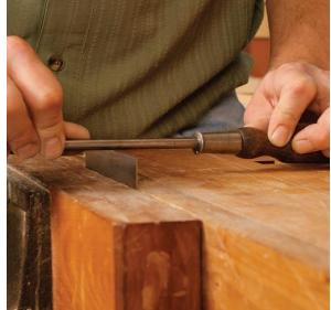
until you feel the burr bite into the wood. It works, but in my experience, it's easier for beginners to start with the scraper held at about 60° and, while pushing, slowly increase the angle until the burr begins to cut the wood. Then push forward in one smooth motion to get continuous, paper-thin shavings.
