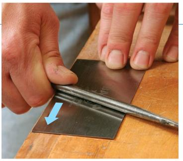
Drawing the burnishing rod over the flat face at a very slight angle extends the corner of the edge out into a ridge.
