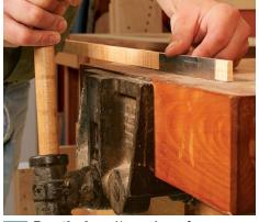
**Turn the burr.** Use a piece of scrap as a reference to set the scraper's edge at a consistent height. Then ride the burnisher's handle along the bench to maintain a consistent angle, and make several firm pushing strokes away from you.
