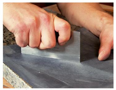
**Remove the wire edge.** A few light strokes on edge should accomplish this. Skewing the scraper to the direction of cut helps keep it square to the sanding surface. This also hones the edge, removing any rough file marks.
