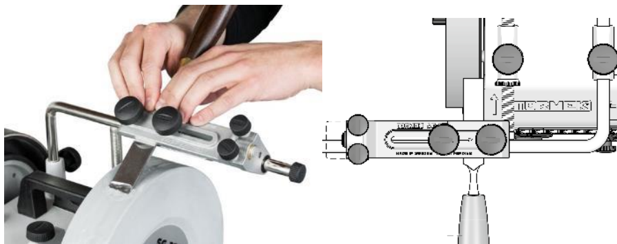
Fig 7 Grinding the primary bevel
