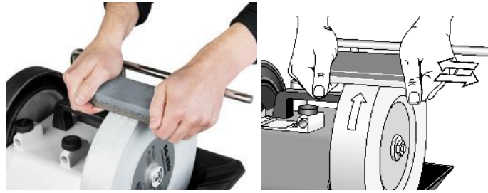
Fig 4 Changing wheel grit level using Stone Grader
