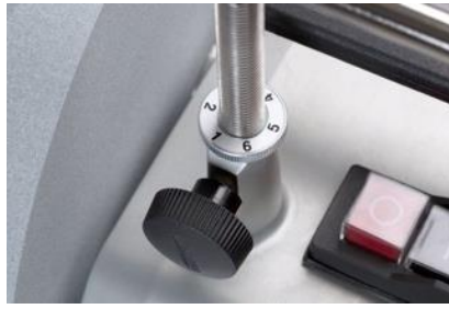
Fig 6b Micro Adjuster Nut
