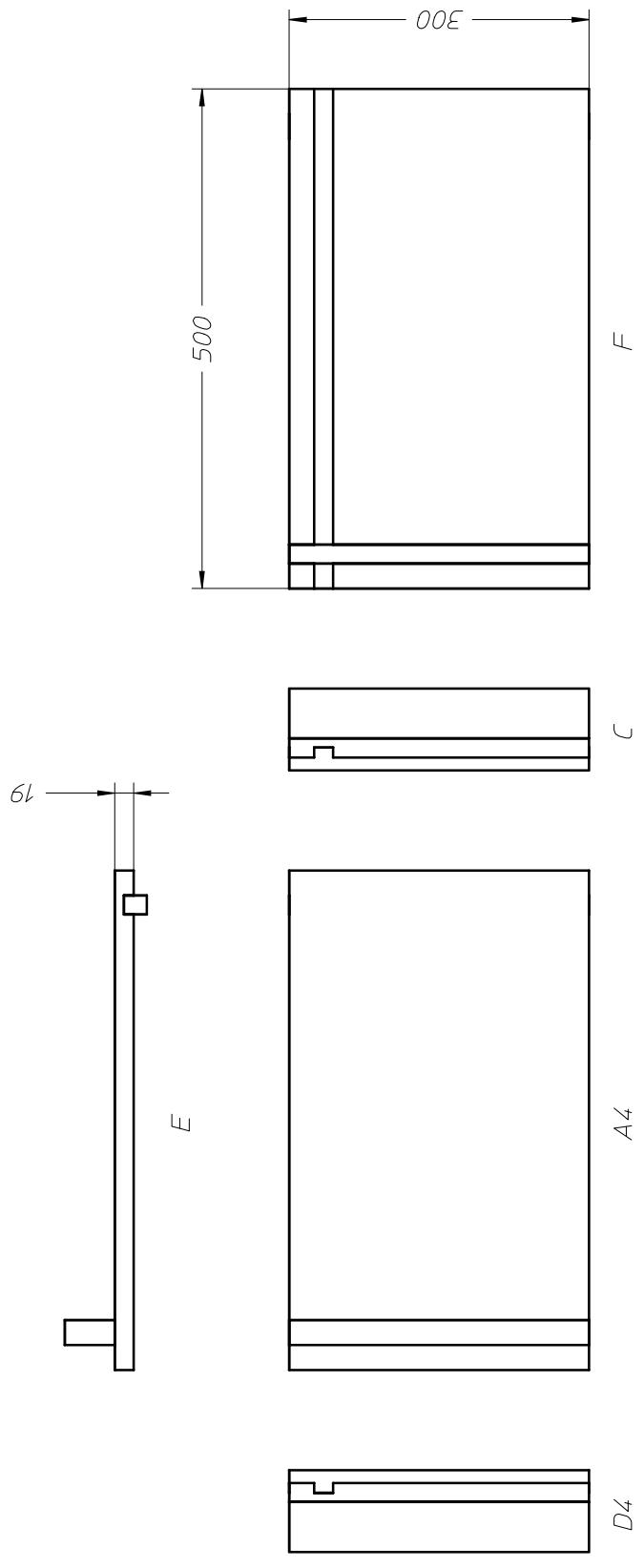
*End Stop Thickness is 2mm less than final timber dimensions in this case
